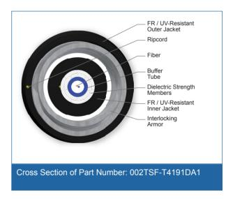
2 F, 50 µm multimode, extended 10G distance (OM4)
