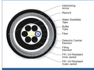
Cross Section of Part Number: 012TUF-T4131DA1
