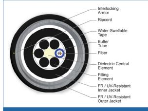
Cross Section of Part Number: 012TUF-T4190DA1
