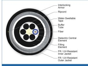
Cross Section of Part Number: 012TUF-T4191DA1
