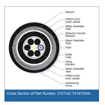
12 F, 50 µm multimode, extended 10G distance (OM4)
