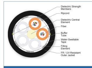
Cross Section of Part Number: 024KWP-T4130D20
