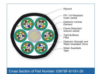
36 F, 50 µm multimode, extended 10G distance (OM4+)
