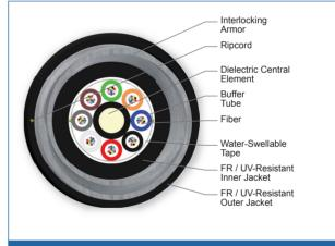
Cross Section of Part Number: 096TUF-T4190DA1
