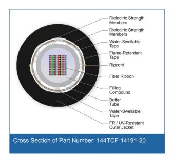
144 F, 50 µm multimode, extended 10G distance (OM4+)
