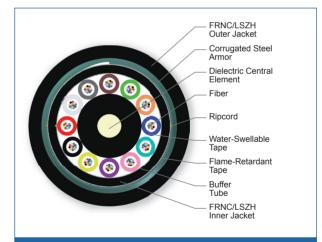
Cross Section of Part Number: 144ZUV-T4101D2N
