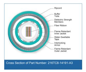
216 F, 50 µm multimode, extended 10G distance (OM4)
