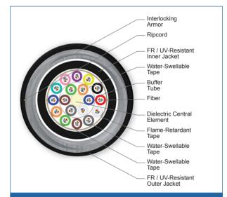
Cross Section of Part Number: 216TUF-T4191DA1
