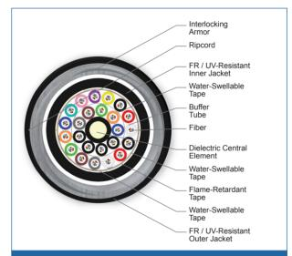
Cross Section of Part Number: 240TUF-T4190DA1
