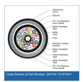
240 F, 50 µm multimode, extended 10G distance (OM4)
