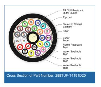
288 F, 50 µm multimode, extended 10G distance (OM4)
