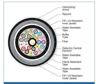
Cross Section of Part Number: 288TUF-T4191DA1
