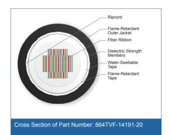
864 F, 50 µm multimode, extended 10G distance (OM4)
